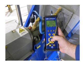
Complete ultrasound solution to manage your acoustic lubrication program and ensure you GREASE BEARINGS RIGHT.
