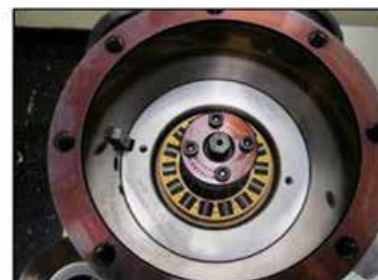
Figure 3. Bearing Setup Inside Test Rig
